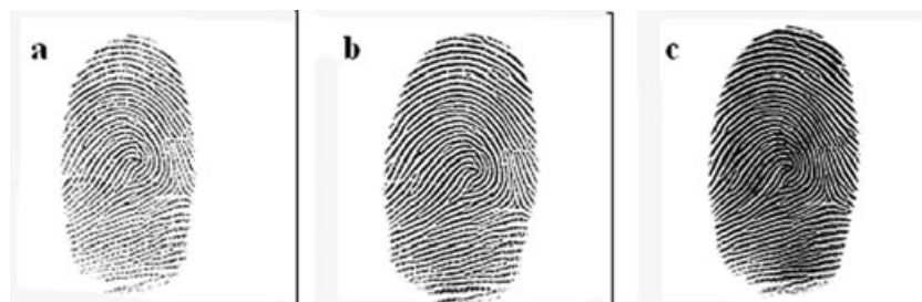
FIG. 2—Results of Livescan images of right index finger at (a) low pressure, (b) medium pressure, (c) high pressure.
