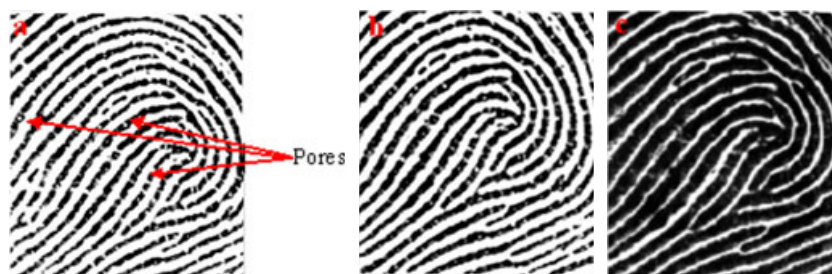
FIG. 5—Pore visibility demonstrated in magnified Livescan images captured at low, medium, and high pressure, respectively.
