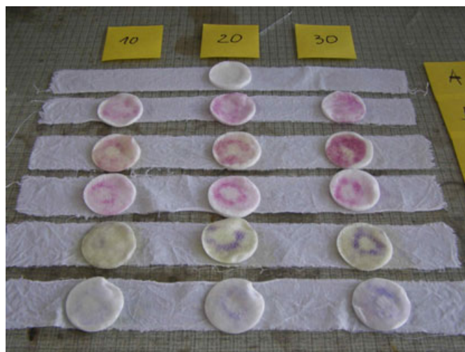
FIG. 4—A complete set of independent tampons with colored traces (left by iron rings) transferred from cotton backgrounds to the tampons. The subsequent rows are corresponding to triazines I to V, respectively. The original contact spots (iron ring-wetted cotton background) on cotton fabrics treated with reducing solution of Sn 2+ prior to the transfer. Room temperature. The single upper sample corresponds to a blind test (no contact with iron ring, treated with same chemical reagents as other spots).
